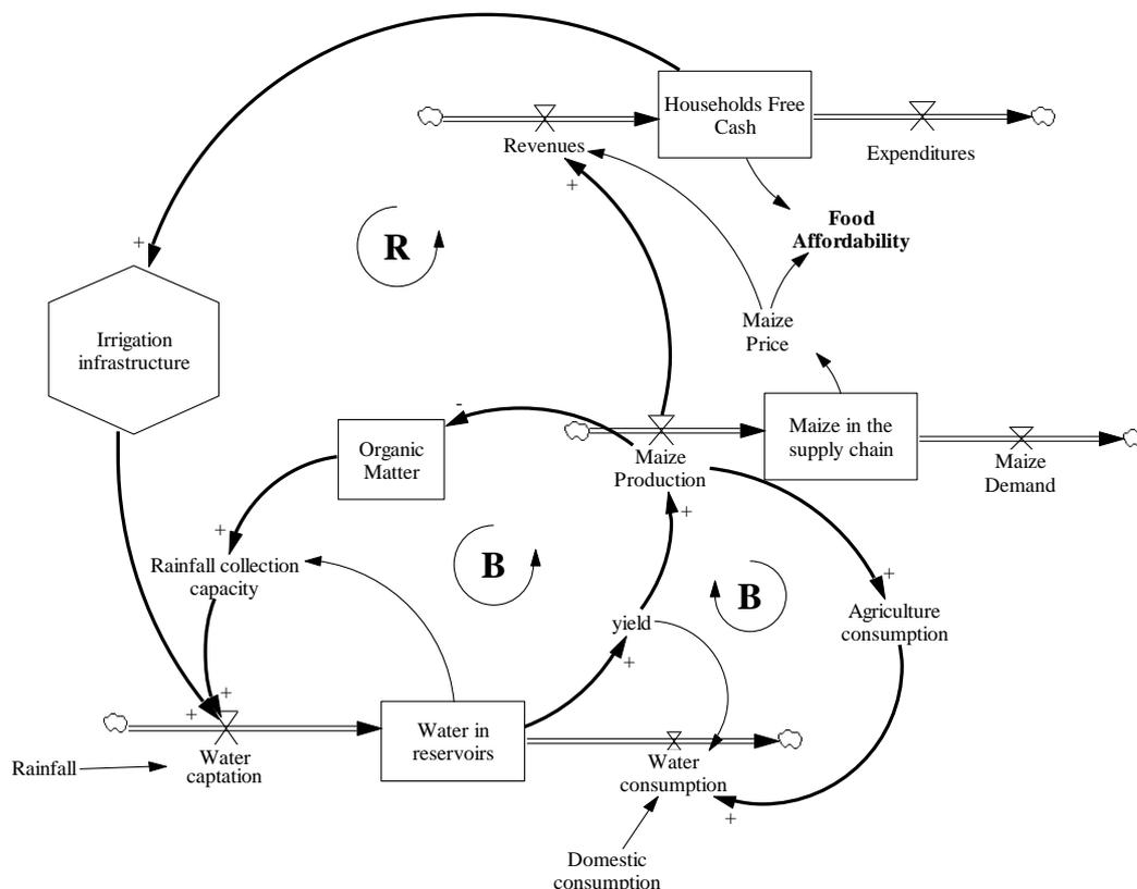
Figure 7: Stock-and-flow diagram representing the performance drivers of maize production
