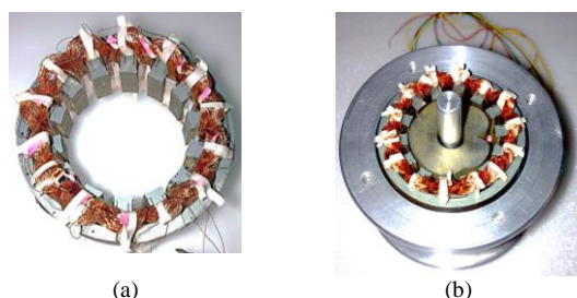
Fig. 10. The prototype multi-turn resolver: (a) the wound stator, and (b) the assembled resolver in its frame
