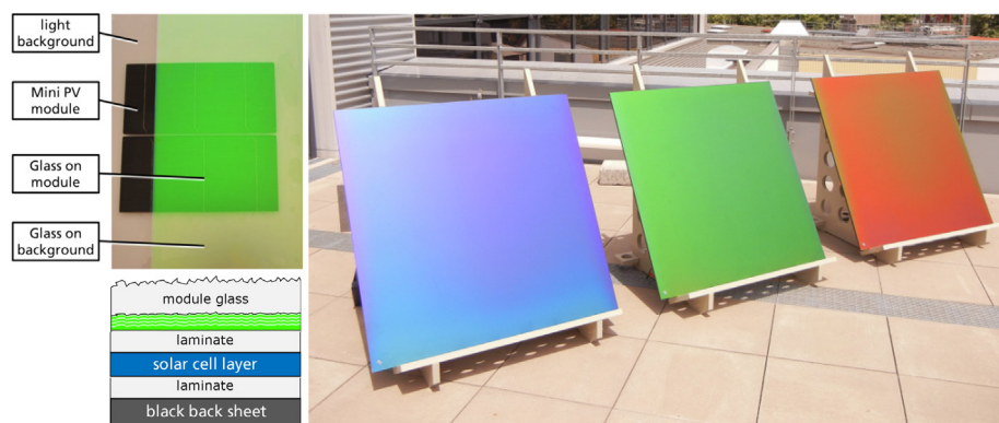
Fig. 24. The figure shows PV modules with the spectrally selective MorphoColor structure located on the inside of the front cover (position 2). The effect is illustrated on the upper left side of the figure, where a black solar cell was placed on a white table and partially covered with a front cover with a green MorphoColor layer. The schematic diagram in the lower left corner shows the structure of a MorphoColor module.
