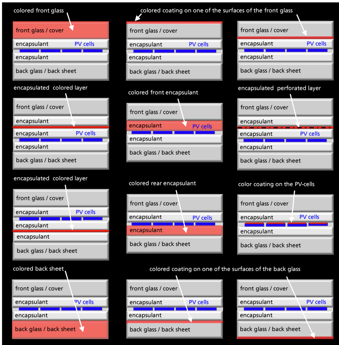
Fig. 23. Colored BIPV module options. The various technical design options are shown in the figure sorted from the outside to the inside, with the outermost layer on top. The colored layer or surface is always highlighted in red.
