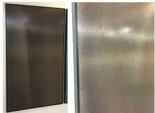
Fig. 11. Solar module with an integrated interlayer (woven fabric) to provide a colored impression (left) and closeup view of the module (right). The woven fabric is placed in front of the solar cell layer and conceals the cells with blackened interconnectors and a black backsheet completely. Depending on the mesh size, the power losses due to the absorption of the woven fabric can be varied but also the appearance of the module changes. A larger mesh size reduces the intensity of the color impression and darkens the overall module. Here, the mesh size results in an absorbance of 35%.
