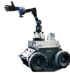
(c) Mobile robot with 3R manipulator
