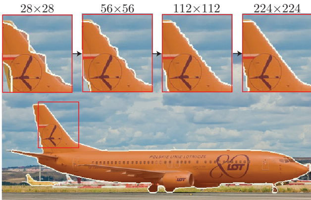
Figure 7: Anti-aliasing with PointRend. Precise object delineation requires output mask resolution to match or exceed the resolution of the input image region that the object occupies.
