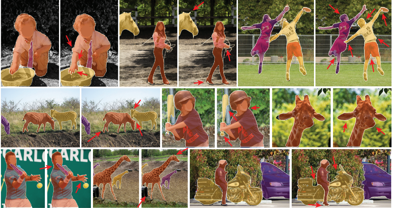
Figure 2: Example result pairs from Mask R-CNN [19] with its standard mask head (left image) vs. with PointRend (right image), using ResNet-50 [20] with FPN [30]. Note how PointRend predicts masks with substantially finer detail around object boundaries.
